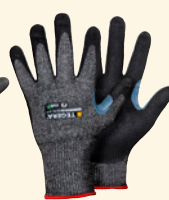
8814 Nitrile, 13 gg, palm-dipped contact heat < 100°C CRF ®
